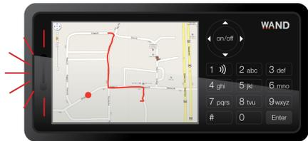
**figure 3:** Using GPRS the device can detect and alert the parent when their child is off the path.
